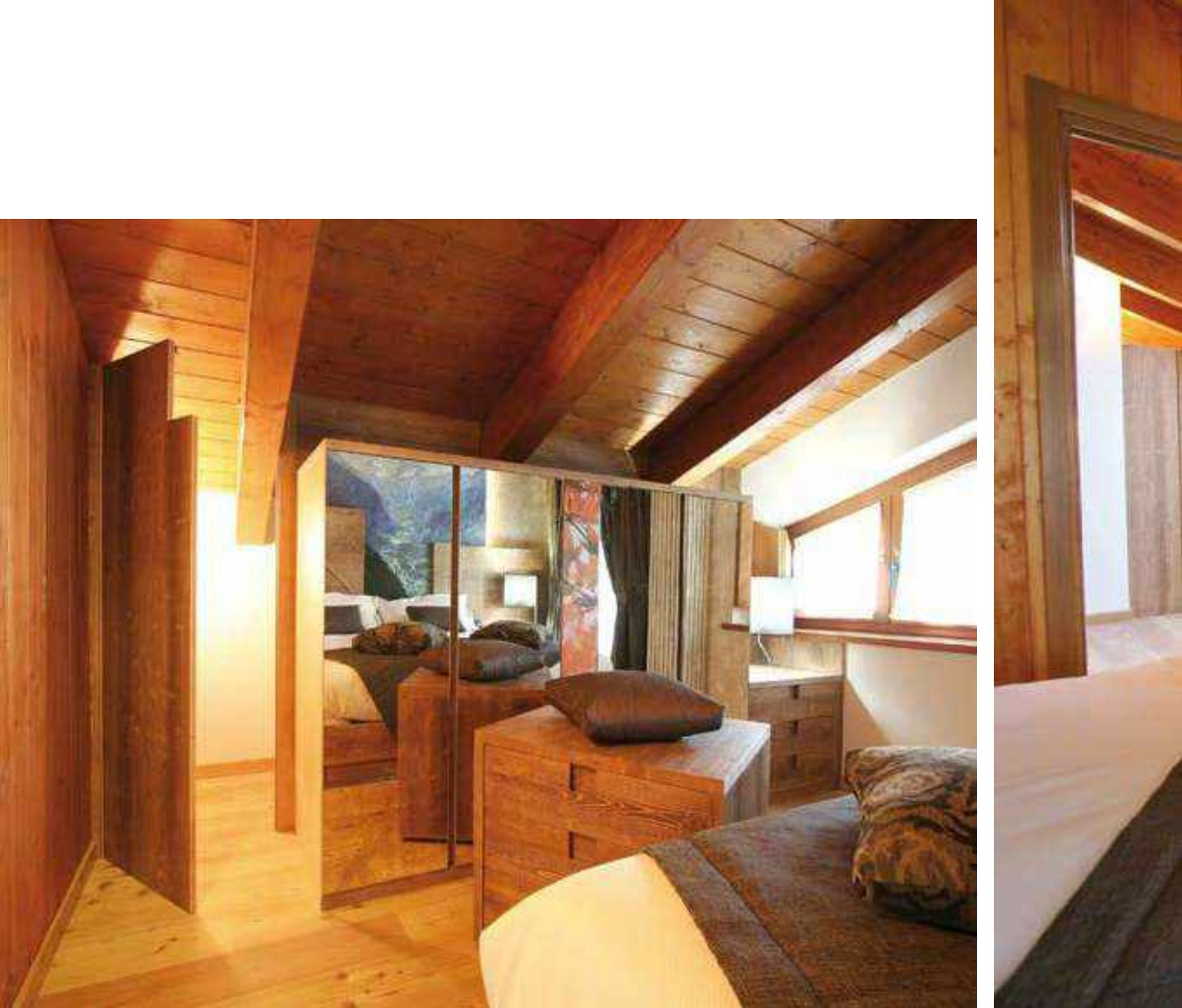
Note how the door was cut to outline the shape of the beam in order to maximize the height of the attic.
